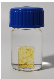
Figure IV-A11 – Swelling in THF for 6 weeks of the reprocessed hybrid dynamic epoxy.
